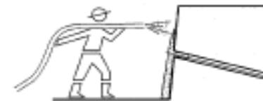
**STEP 4. Place Drainage Strips, Initial Shotcrete Layer & Install Bearing Plates/Nuts**
